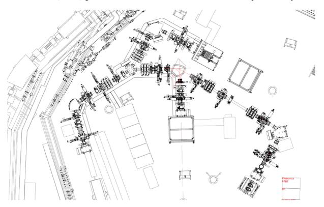
Two sources are installed in the existing LEBT. One is used to produce protons (O1) while the other for the production of carbon ions (O2). A third source (O3) will be installed in the LEBT CNAO with the aim of producing new ionic species both for clinical purposes (Helium, Oxygen) and for experimental purposes (Iron, Lithium).
